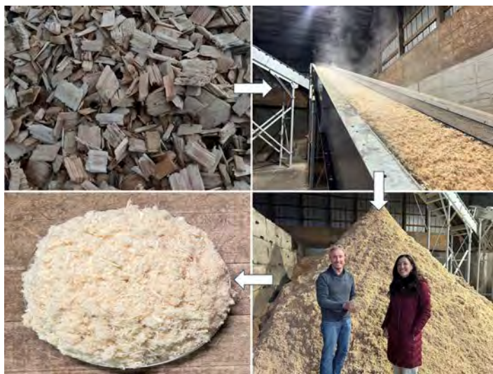
Figure 1. White pine chips being extruded into wood fiber growing media at P.R. Russell in Brentwood, NH.
