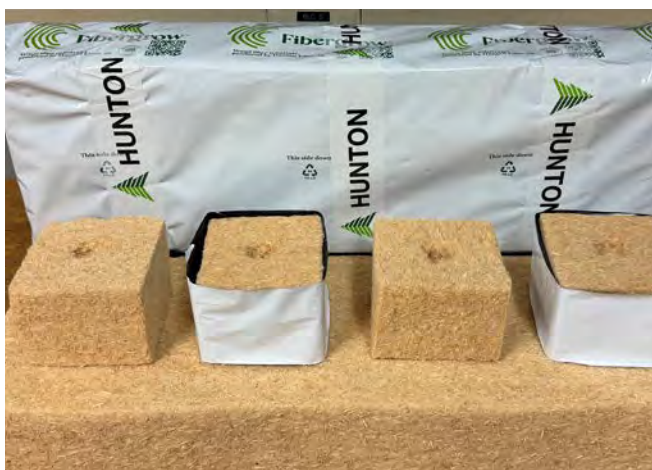
Figure 3: Slabs and blocks of an engineered wood fiber (Fibergrow) produced by Hunton in Norway.
