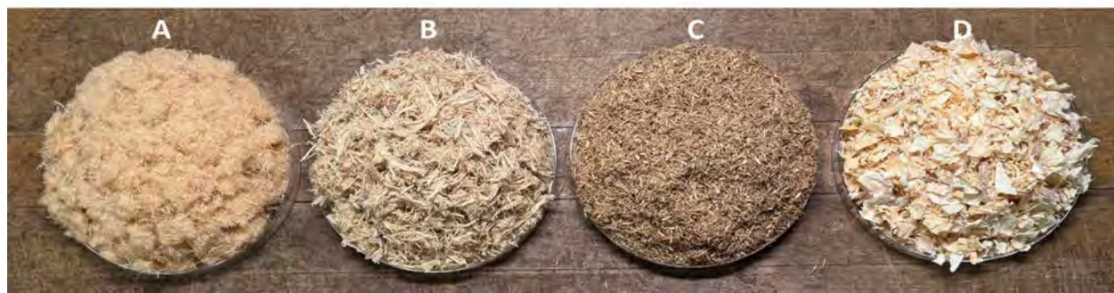
Figure 1: Manufactured types of wood substrate products: (A) disc-refined, (B) extruded, (C) hammer-milled, and (D) shavings. Photo: Brian Jackson
