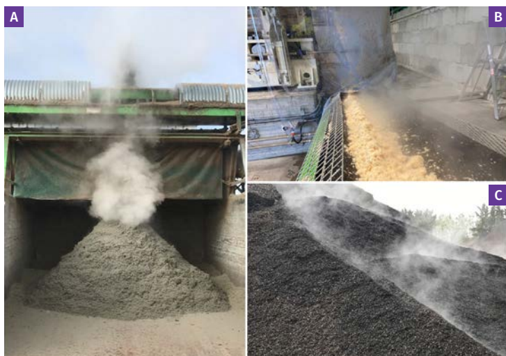
Figure 2. Steaming or heating during or after processing of some organic substrates is an important step in preconditioning materials before use.
