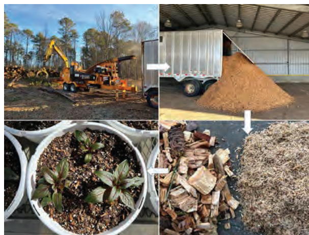
Figure 2. This collage shows the process of harvesting, chipping, milling, and aging pine trees for use as substrate components.
