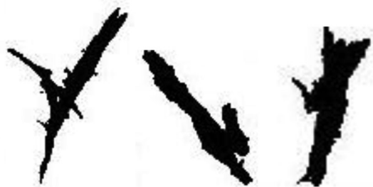
FIGURE 3 Wood fiber particles showing convex parts explaining discrepancy in various diameters assessing the width.
