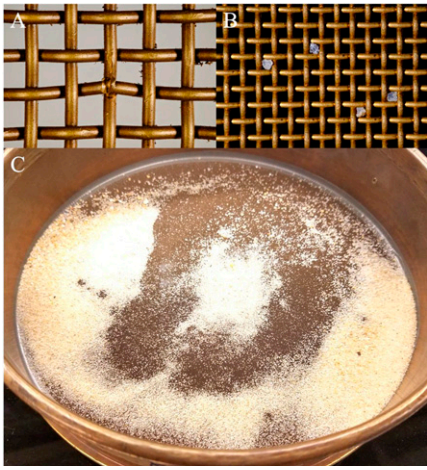
Fig. 2. Variability in aperture size and obstructions within apertures may result in errors when using sieve for particle size analysis. (A) Damaged woven wire screens can decrease or increase aperture sizes beyond that of the tolerated deviation allowed by American Society for Testing and Materials (ASTM) Standards. (B) Entrapped particles will diminish the percentage of open apertures. (C) Raised areas or depression on a sieve screen will result in poor sample distribution (photo credit: David Suchoff).
