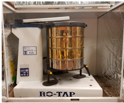
Fig. 1. A nest of sieves (brass) and pan (steel) agitated by a Tyler Ro-Tap machine.
