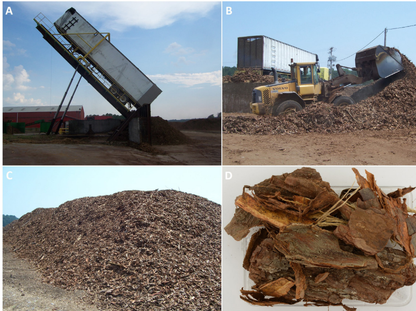
Figure 1: (A) raw pine bark from lumber mills is (B) delivered to substrate processing facilities and often (C) inventoried in piles/windrows in its (D) raw form before being milled into smaller particle sizes at some future time.
