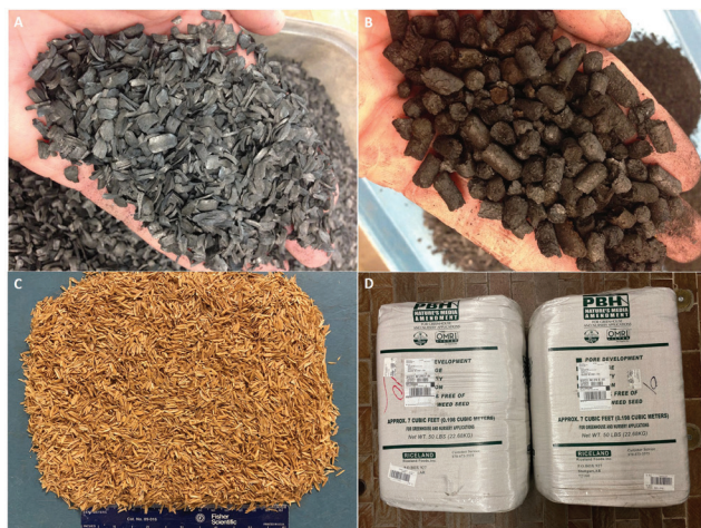
Fig. 4. Miscanthus biomass can be processed in different ways (extruded, disc-refined, and hammer milled) to create unique fibrous materials for potential use as substrate components.
