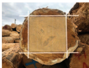
Figure 2. The edges (side planks) are removed from sawlogs at the mill. The inside "heartwood" of the tree (shaded portion) is used for lumber, poles, etc. while the removed outside "sapwood" edges can be chipped and used as feedstocks for making substrates.
