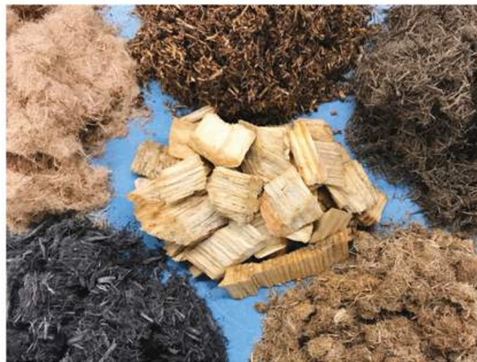
Figure 1. Wood substrate components vary in their manufacturing processes, particle size and shape, and color, as well as the ability to be easily mixed.
