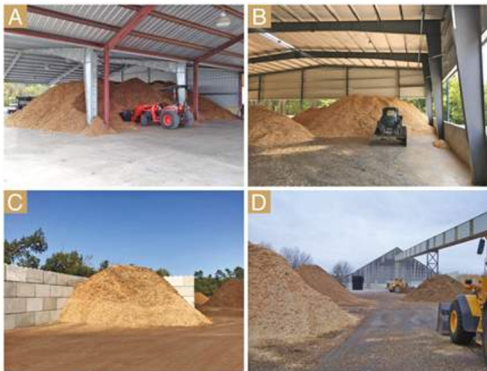
Figure 2. Wood chips to be hammer-milled should be stored under shelter (A and B) to prevent being rained on, while wood chips destined for other processing methods can be left outdoors (C and D).
