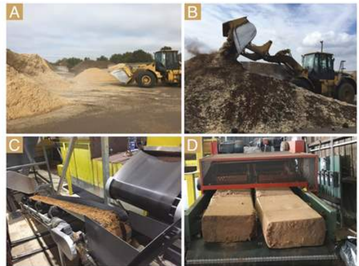
Figure 4. All wood substrate materials cannot be blended with other materials the same way. Different techniques—including pad mixing with loaders, conveyor mix lines or specialized fluffing/blending equipment—are among the options for mixing.
