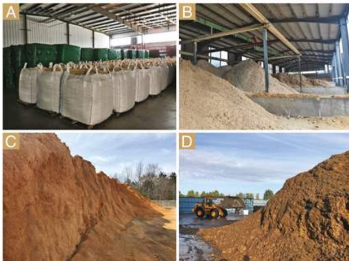
Figure 3. Once processed, some wood components should be stored in totes (A) or under shelter (B) to keep dry, while other products can be left outdoors (C and D).
