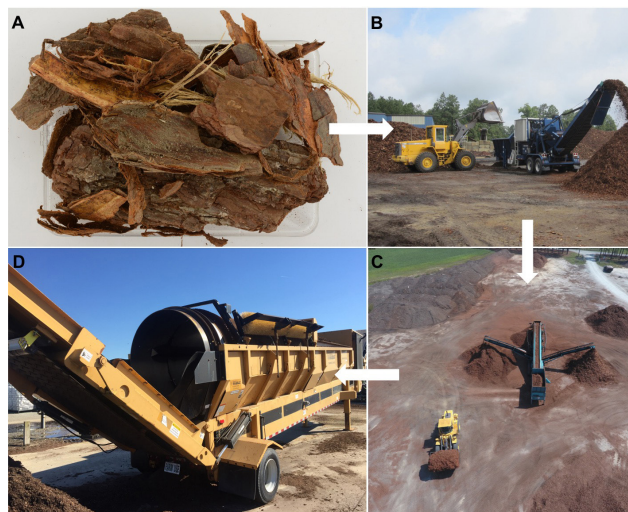
Figure 4: Raw bark removed from freshly harvested trees [A], is delivered from sawmills to bark processors for further grinding [B], sizing and windrowing [C], and screening to create specific substrate products.
