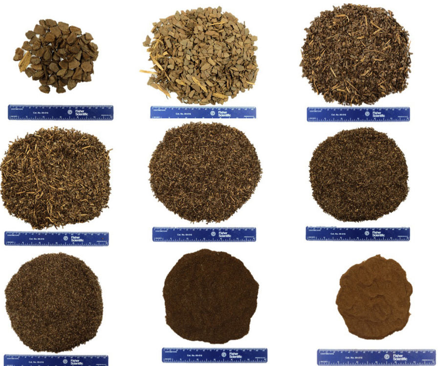
Figure 5: Deconstruction of a nursery bark substrate illustrates the particle size (and shape) range that can be created to yield specific physical and hydrologic properties.
