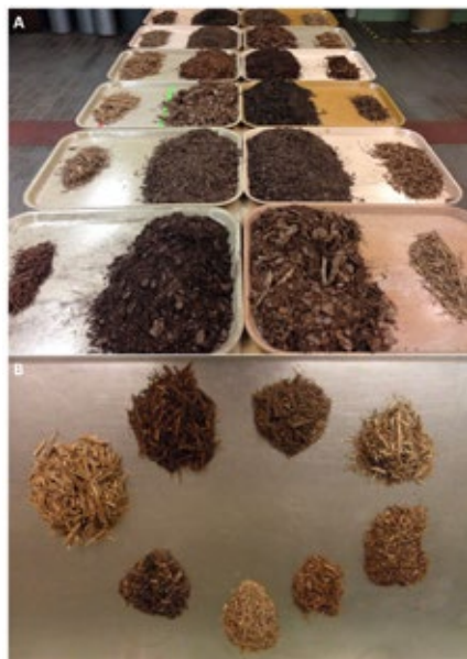
Figure 3: Twelve pine bark substrates acquired from multiple suppliers that have had the white wood hand-extracted to determine percent (A) and grouping of 8 samples of the extracted white wood showing variation in particle size.
