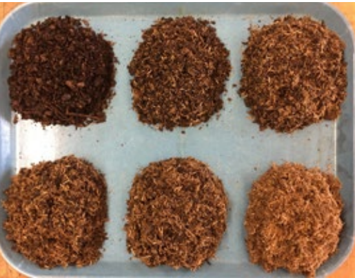
Figure 5: Processed pine tree substrate blended with aged pine bark at 0, 20, 40, [top row left to right] 60, 80 and 100% [bottom row left to right].
