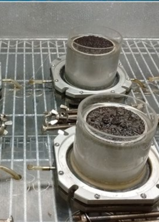
Figure 3: Laboratory analysis of aged pine bark substrates are used to quantify changes in hydration/wettability (A-B), saturated hydraulic conductivity (C), physical properties and water retention/release properties (D).
