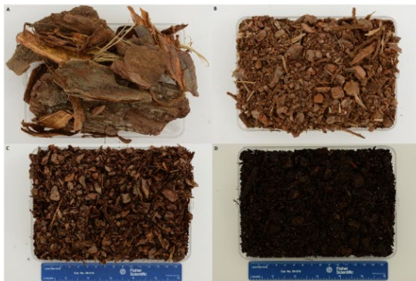
Fig. 1: Raw pine bark after being removed from harvested trees (A), hammer-milled fresh bark (B), bark after one month aging in windrow (C), and bark after eight months of managed aging in windrows (D).
