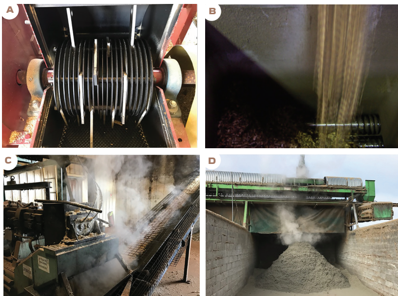
Fig. 2 Common machines used to make wood substrate products include hammer mills (A), single or twin-screw extruders (B), and twin-disc refiners (not shown) which produce varying amounts of heat (C-D).
