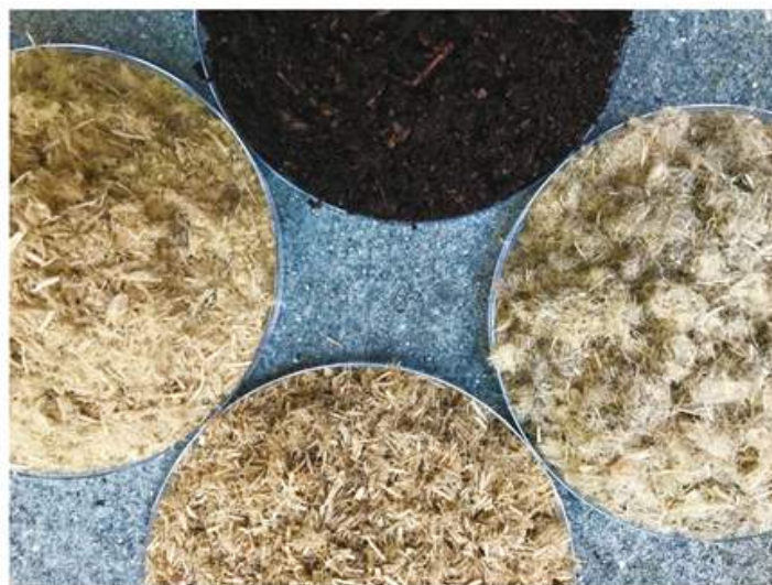
Figure 1. Substrate materials tested for hydration efficiency were (clockwise from top) peat moss, ForestGold, Pine Tree Substrate and HortiFibre, which represent three different processing methods.
