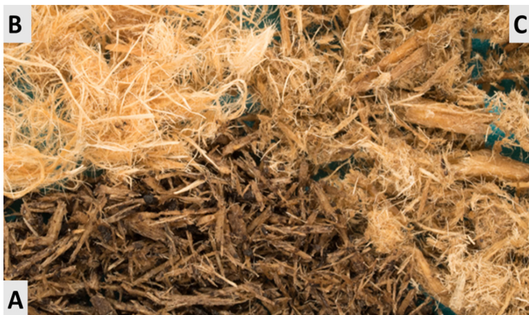
Figure 1. Three wood fiber substrates tested for physical and wettability properties, wood fiber 1 (A), wood fiber 2 (B), wood fiber 3 (C).
