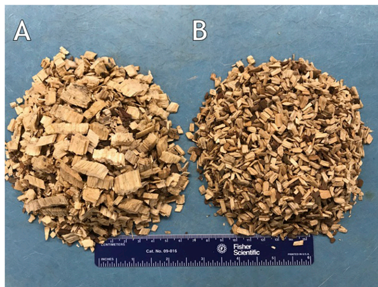
Fig. 1. Depiction of large loblolly pine wood chips (PWCs) produced by processing delimbed logs (with bark intact) through a chipper (A) and after 2 d, wood chips were hammer-milled through a 0.25-inch (6.350-mm) screen resulting in smaller PWCs (B).
