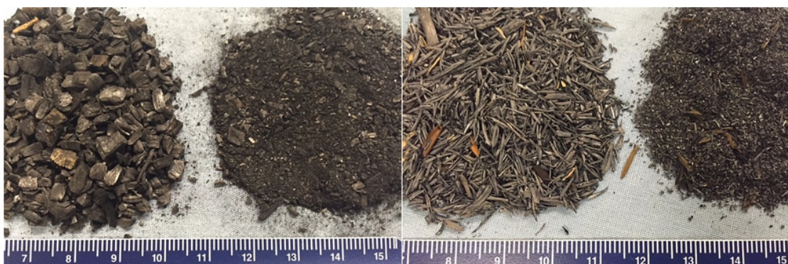
Figure 1. (Left) Comparison of biochar produced from pine wood (loblolly; Pinus taeda ), that was then ground to <2-mm size (right; PBC p ). (Right) Comparison of biochar produced from rice hulls, that was then ground to <2-mm size (right; RBC p ). Centimeter ruler shown in both pictures for size comparison.
