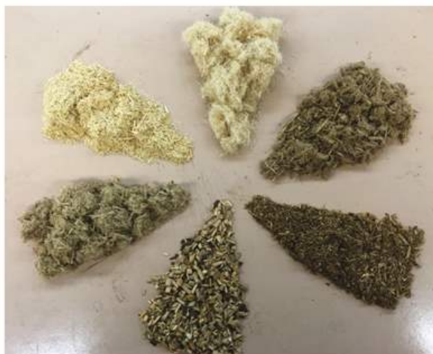
Figure 1. Wood substrate components vary in particle size and shape as a result of different manufacturing methods.
