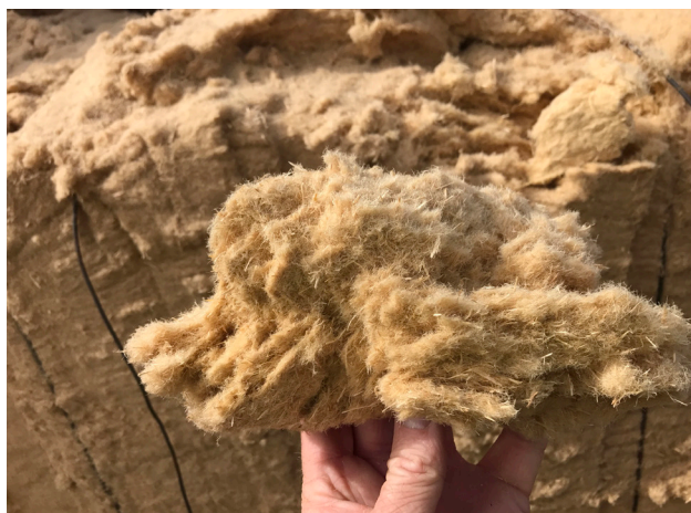
ABOVE: Fig. 3. Wood fiber produced with twin-screw extrusion can be easily used (typically blended with peat moss) in loose-fill containers for vegetable production.
