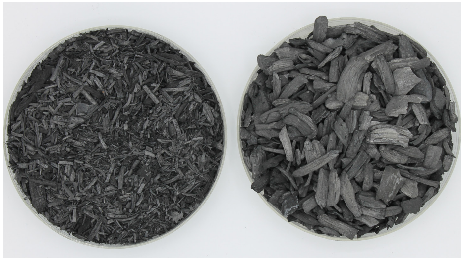
Switchgrass biochar (left) and hardwood biochar (right), both produced at approximately 1,000 C.
