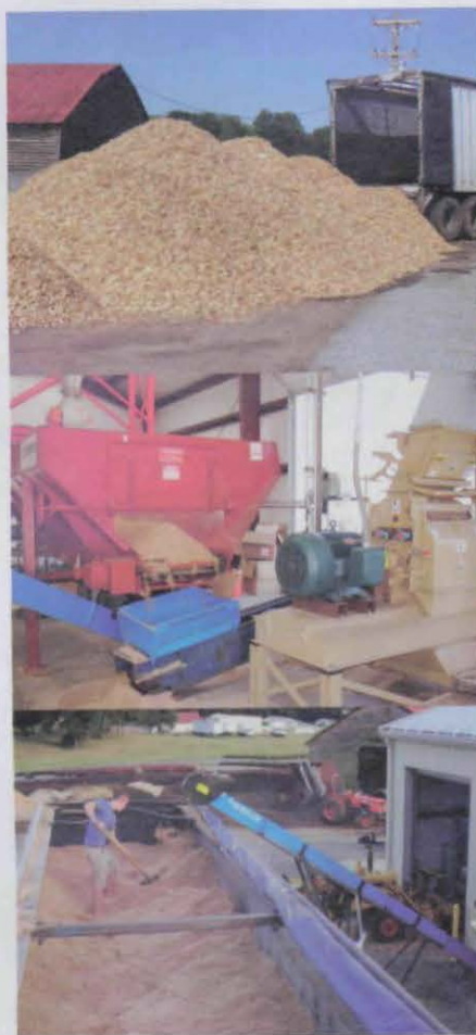
Loblolly pine trees have been harvested and are ready for transport to a processing facility. The pine trees are then chipped and ground in a hammer mill to produce pine tree substrate. The substrate can then be transported, stored or used immediately.
