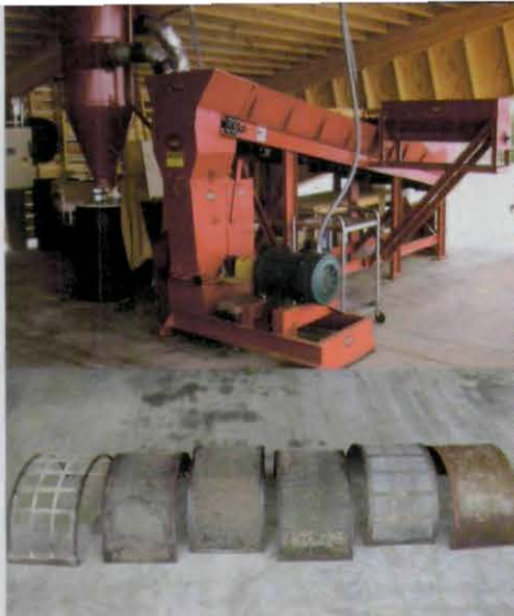
A hammer mill can be fitted with different-sized screens to grind coarse wood chips into any particle size to produce a substrate with physical characteristics similar to pine bark or peat-based mixes.
