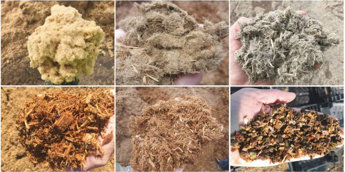
Figure 1. Several wood substrate materials from European manufacturers show variations in particle size and structure.
