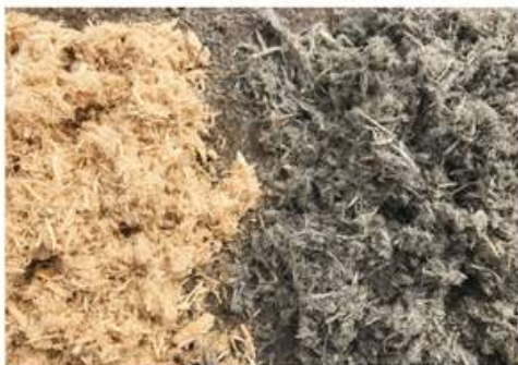
Figure 4. Coloring of wood fiber (with charcoal) is easily done during the mechanical processing of wood chips.
