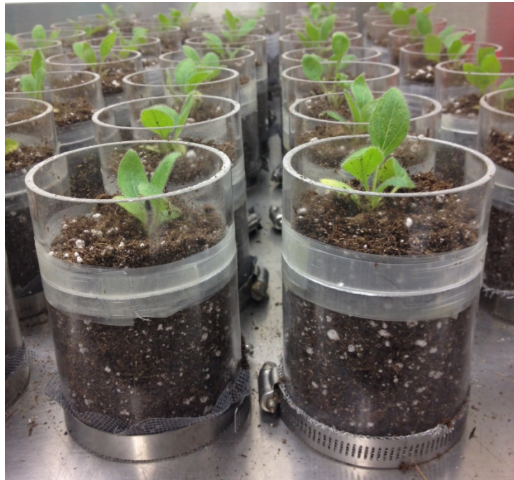
Fig. 2. Planted Rhizometers, without foil covers so that the clear sides and the attached collar are visible. The bottom ring is holding a screen to allow for drainage.
