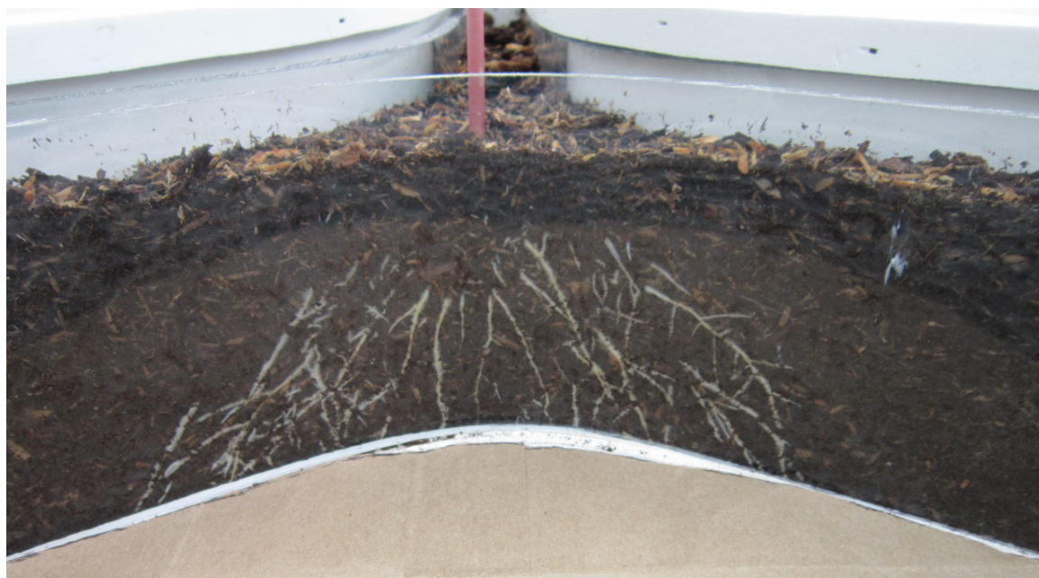
Fig. 1. A planted mini-Horhizotron, seen here with two arm faces visible (without the shade panel) and the root branching/architecture can be observed. Shade panels are in place against the other arm sections.
