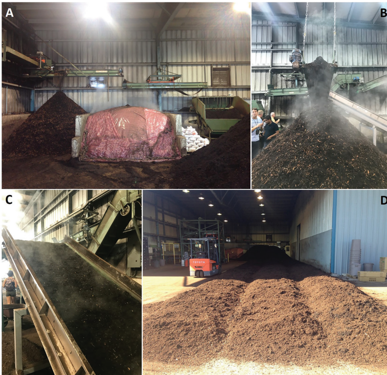
Fig. 4. Some greenhouse operations have implemented successful substrate recycling programs that include (A) grinding rootballs followed by steam sterilization of processed substrate. The steam heated processed substrate materials (B and C) can then be aged or stored until being incorporated back into the crop production cycle.
