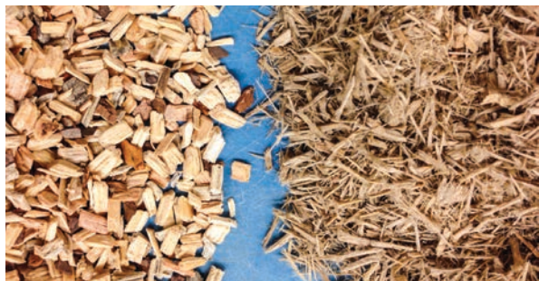
Figure 2. Comparison of pine wood chips (PWC) engineered to be used as an aggregate (right) and shredded pine tree substrate (PTS) engineered for use as a peat-extender (left). Both wood components were processed from similar-aged trees, harvested at the same time but processed differently to yield specific desired products.
