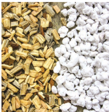
Figure 3. Comparison of pine wood chips (left) engineered to have the same particle size as this coarse-grade of perlite (right).
