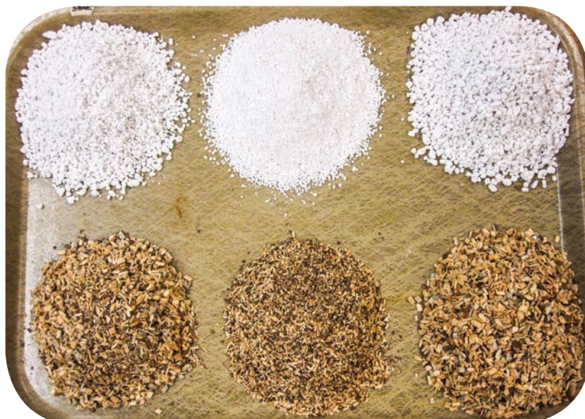
Figure 4. Different sizes of PWC can be created to have the same particle size as different grades of perlite. Coarse particles on the right, medium particle size on the left and a mix of the two sizes in the middle.
