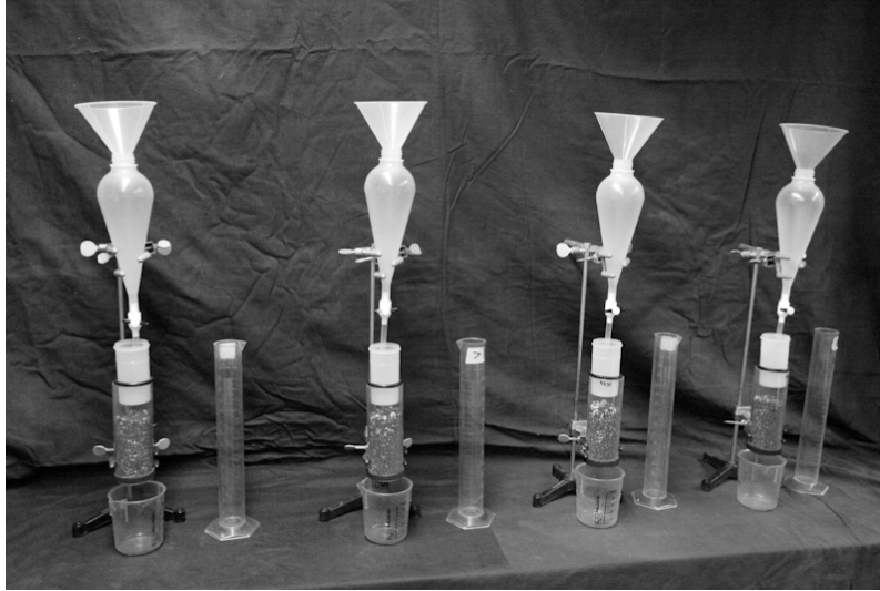
Fig. 1. Hydration unit setup for testing with four replications.
