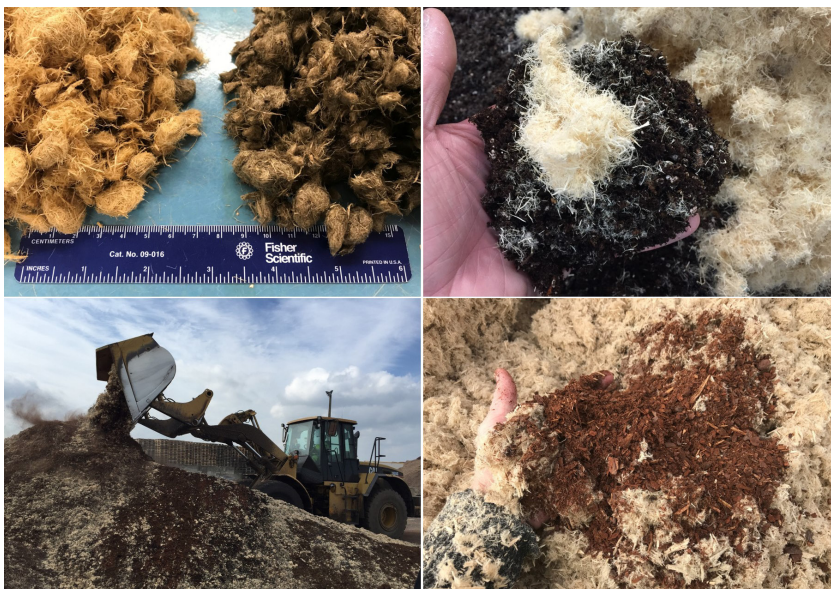
Figure 2. Blending some wood components with peat, bark, or other materials can require specialized equipment while other wood products can be easily and thoroughly blended with existing machinery or methodology.
