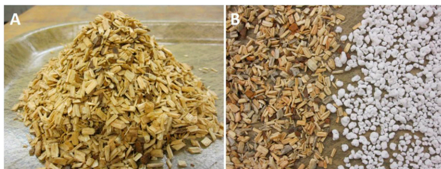
Fig. 1. (A) Harvested loblolly pine logs were chipped in a wood chipper resulting in large wood chips [ 1.0 \times 0.2 \times 1.0 cm (length \times width \times height)] before being milled through a 1/4-inch (6.35 mm) hammer mill screen resulting in (B) smaller pine wood chip (PWC) aggregates that are square/blockular in nature and contain little dust or fibers and are similar in size to horticultural grade perlite; 1 cm = 0.3937 inch.
