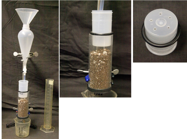
Figure 4. The parts of the wettability unit. Left/ A whole unit assembled; center: the diffuser fitted with the O-ring on top of the substrate; right: the bottom of the diffuser with 5 holes drilled to allow for more equal flow across the substrate surface.
