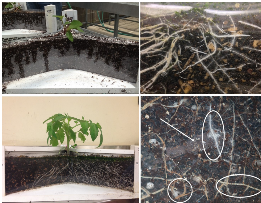
Figure 2. The mini-Horhizotron. Clockwise from top left: water penetration, root exploration and branching, disease effects of healthy (circles) and damaged (arrow) roots, disease spread (inoculated from left side of image). (Image originally published in Judd et al., 2014b).
