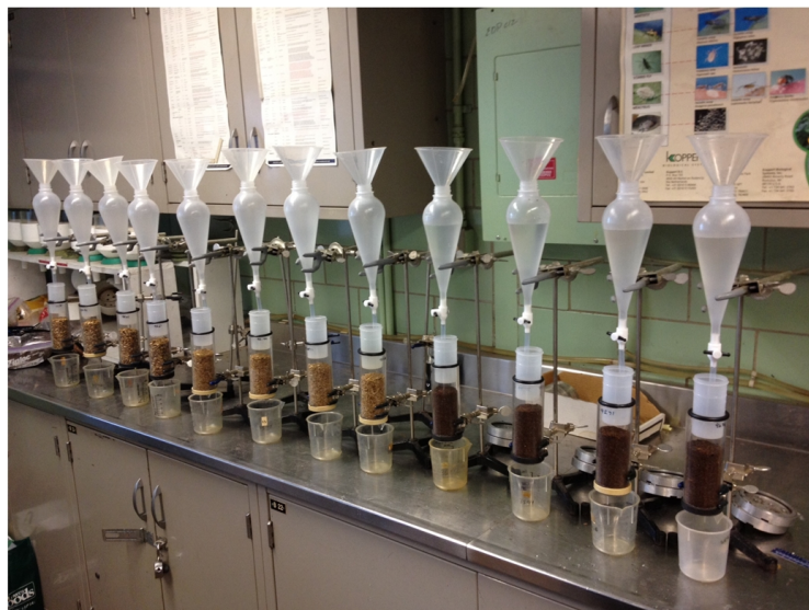
Figure 5. Wettability units being used to generate a hydration curve for three different materials.
