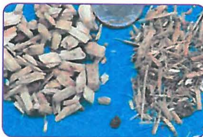
Figure 1. Comparison of pine wood chips (PWC) engineered to be used as an aggregate (on left) and shredded pine tree substrate (PTS) engineered for use as a peat-extender (right). Both wood components were similar aged trees, harvested at the same time, but processed differently to yield specific desired products.
