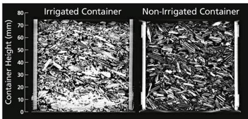
Figure 2. Pine bark cores were analyzed before and after irrigation. White or light grey objects indicate the presence of solids and water. Black spaces indicate air-filled regions.
