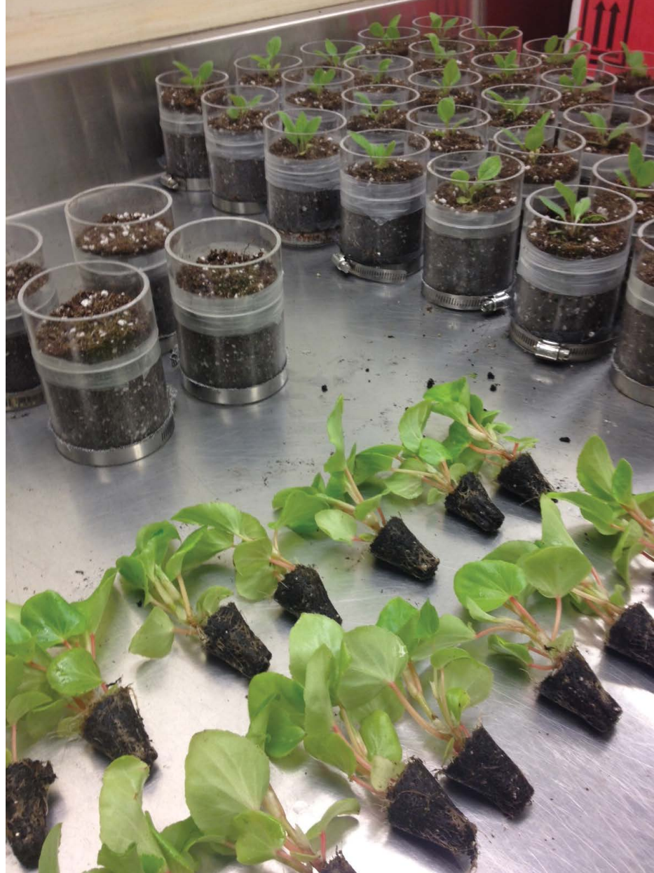
Above, plugs are readied for planting in rhizometers for growth study and comparisons. Left, To construct the Rhizometer, clear, cylindrical Plexiglas tubes were cut, and a collar was attached to the top of the core with parafilm. The collar extension is attached to the top of the core to aid in packing the core; it also allows extra space for planting a plug. A 20-mesh fiberglass screen was cut to fit the bottom of the core and attached with a hose clamp.
