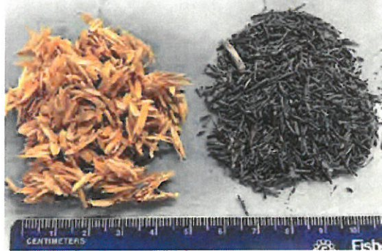
TOP: Pine wood chips and pine biochar; Bottom: rice hulls and rice biochar used in studies at NC State University.
