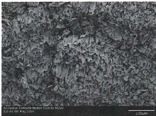
Magnified side view of a pine biochar particle
