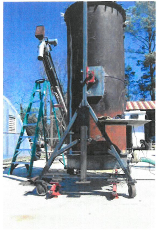
Top-lit updraft (TLUD) gasifier
