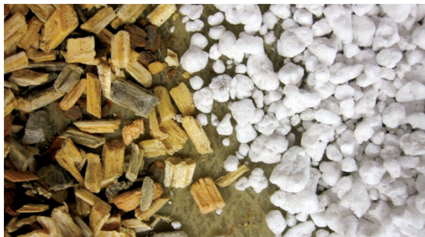
Figure 2. Comparison of pine wood chips (left) that have been engineered to have the same particle size as this coarse-grade of perlite (right).
