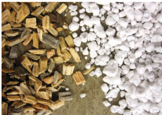
Figure 2. Comparison of pine wood chips (left) that have been engineered to have the same particle size as this coarse-grade of perlite (right).
