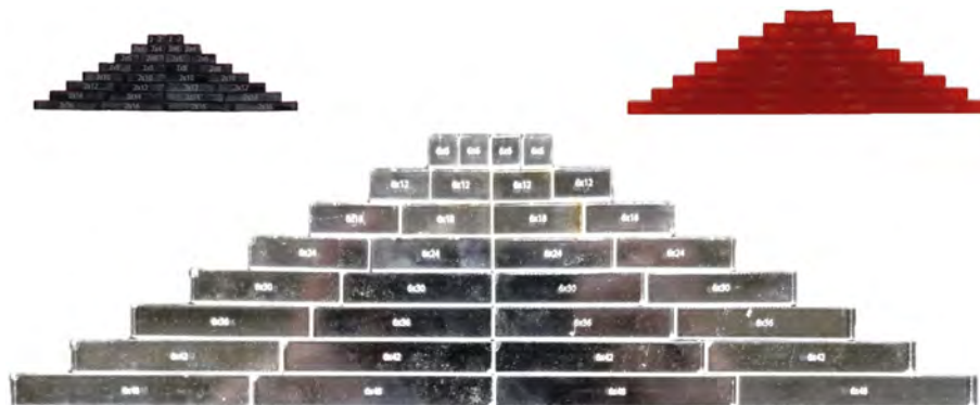
Fig. 1. Acrylic sheets were cut into three size classes of particles: 2-mm (top left), 3-mm (top right), and 6-mm (bottom center). Eight length to width ratio particles were cut in each size class from 1:1 to 8:1. The sizes were etched onto each particle for ease of identification and separation during analysis.
