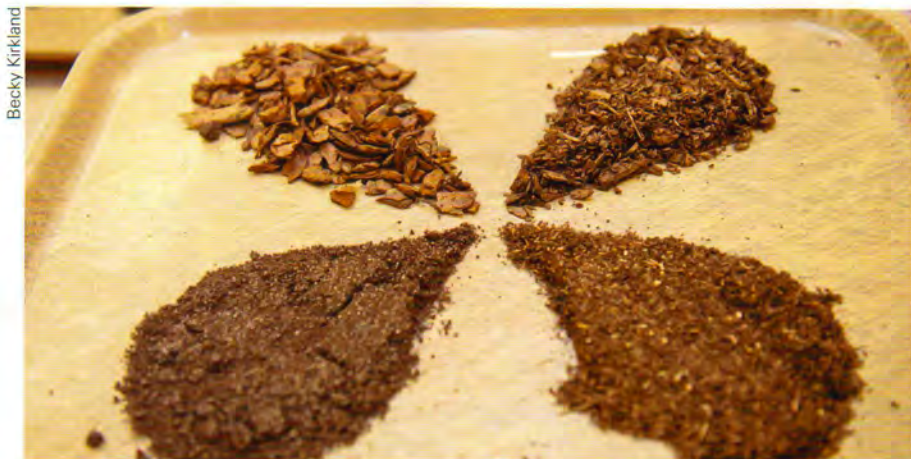
Wood chips (right) fed into the hammer mill will be pulverized and rendered into desired particle sizes via chosen screens. This process yields the varieties of substrates (above) to suit potting purposes and geographic needs.
