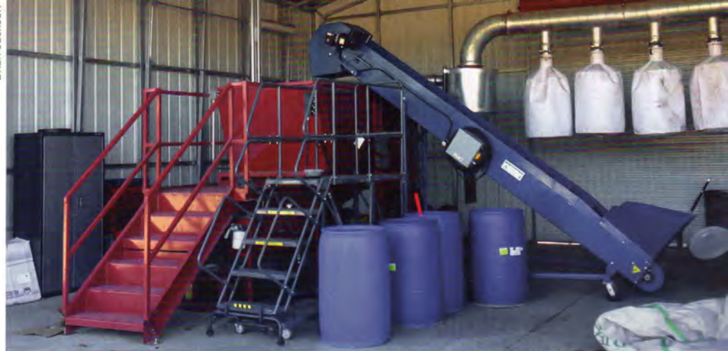
The SPARC enables large-scale processing of organic materials – such as wood, bark, grasses, tobacco stalks – that can be used in developing the next generation of potting soils. The SPARC also facilitates lab activities and, with the creation of new products, can be an economic stimulus.
