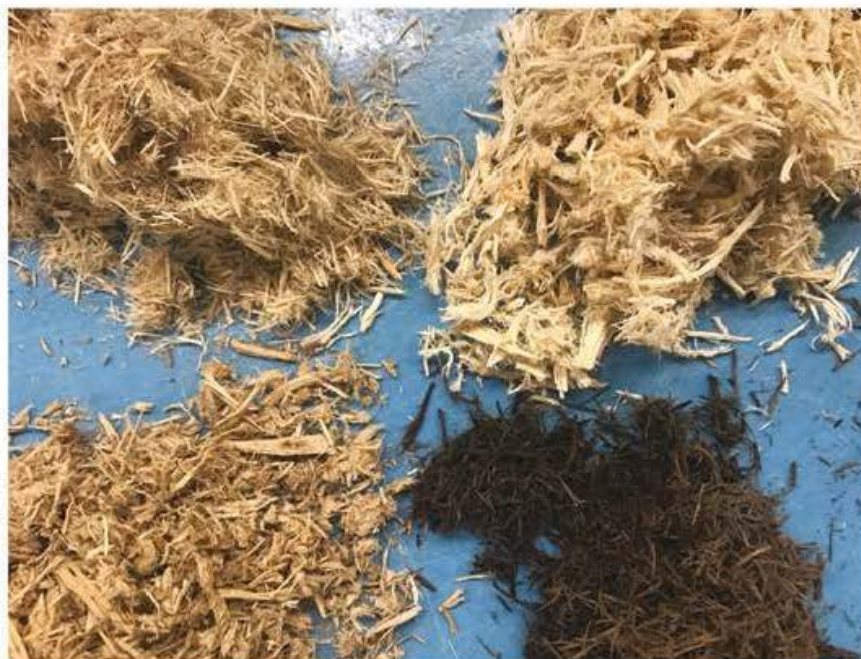
Figure 1. Different types of commercial wood substrate materials are available in North American and European markets, most being fibrous in texture/structure.
